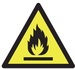
Caution: Risk of fire/ flammable materials
