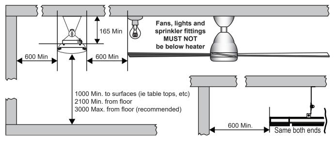
Minimum clearances when mounting the heater at an ANGLE TO A CEILING.
