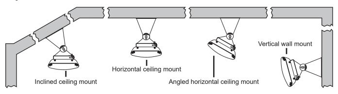
The ideal mounting position is directly above the area to be heated with a longitudinal orientation and facing vertically downwards. If this is not possible, the heater(s) can be mounted on a wall and angled downwards. For this application ensure the mounting height is within 2.1m to 2.7m.
