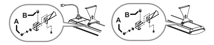
Depending on material and design of ceiling structural elements, the heater must be secured with the correct fasteners. Refer to table below for weight of the heater. The installation location MUST be able to hold 5 times the weight of the heater.
