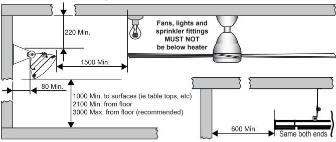
Minimum clearances when mounting the heater parallel with **A CEILING**.
